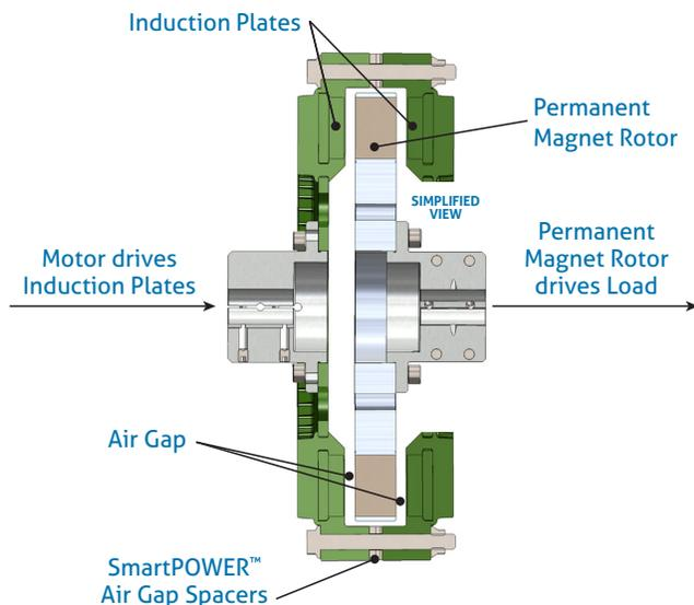
The induction rotor portion of the FSC, representing about 70% of the product's total weight, is typically mounted to the motor shaft. The two induction rotor plates are held together by thru-bolts. The separate aluminum rotor with embedded magnets is positioned between the two induction plates.
