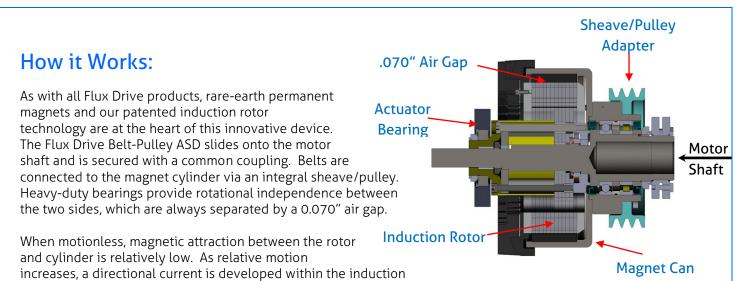
rotor. This current creates a magnetic coupling effect that builds rapidly across the air gap until the drive begins to rotate the load. The time between full "slip" at start-up and full load speed is the soft-start period. This is typically 5-10 seconds but can be adjusted. At full engagement, the device operates at 98.5% efficiency. To adjust speed, the rotor is moved axially in and out of the magnetic cylinder, weakening or strengthening the magnetic field.
