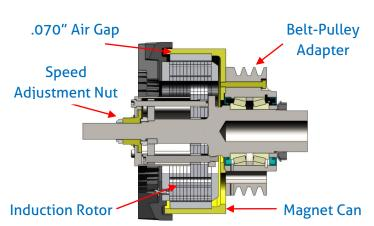
motion increases, a directional current is developed within the induction rotor itself. This current creates a magnetic coupling effect that builds rapidly across the air gap until the drive is able to rotate the load. The time between full "slip" at start-up and full load speed is the soft-start period – typically 5-10 seconds. At full engagement, the device operates at 98.5% efficiency.
