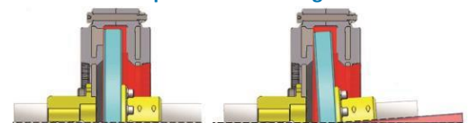
Air Gap Tolerates Misalignment
